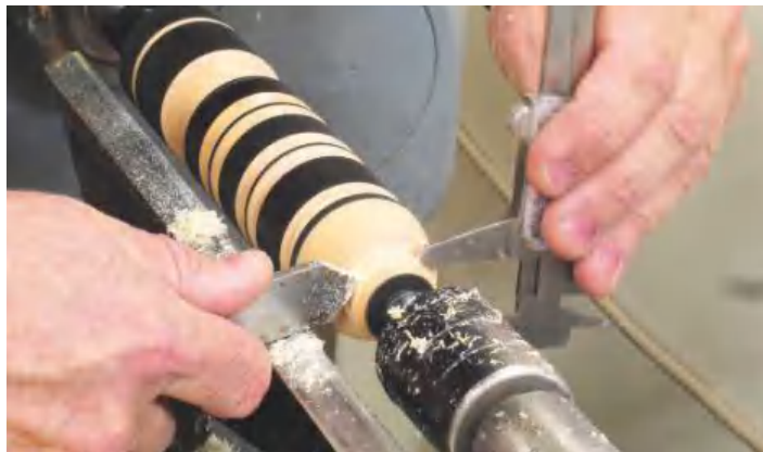
▲ Pic.5 Sliding the tool along the rest and taking a small cut will leave an acceptable finish on most timbers
